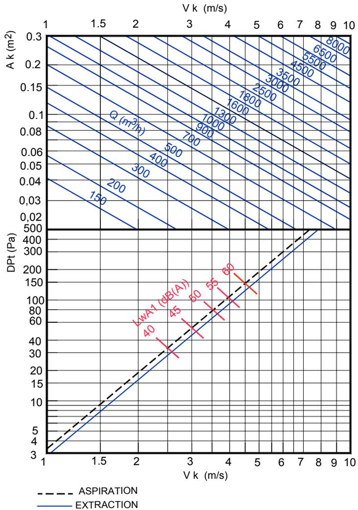
$$V_k \text{ (m/s)} = \frac{Q \text{ (m}^3 \text{/ h)}}{A_k \text{ (m}^2\text{)} * 3600}$$
